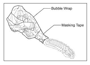
While still inside the vehicle, use bubble wrap and masking tape to cover and protect the sensor.
