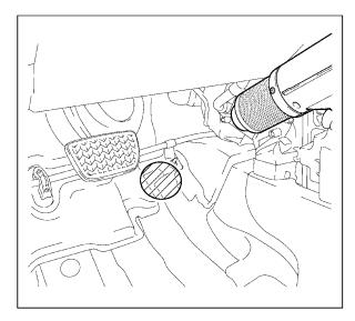
2. Using a hair dryer or low temperature heat gun, warm up the sound deadening material until it becomes soft.
